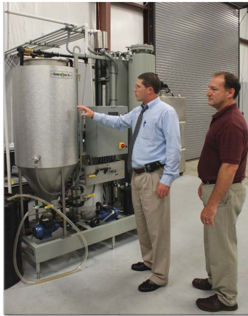
Calhoun County Engineer Brian Rosenbalm, CEA, and Project Engineer Jeff Clendenning demonstrate the equipment necessary for turning used vegetable oil into biodiesel fuel.
